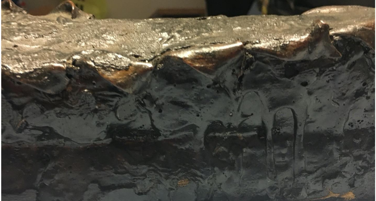
Fig. 1 – Photograph showing the drip lines caused as the molten resin and beeswax emulsion settled prior to solidification.
