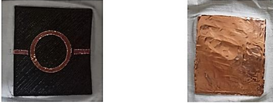
Fig. 2: Front and bottom side of a ring resonator
